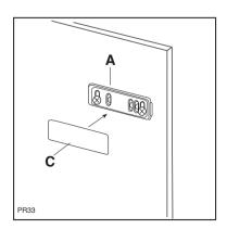
Open the appliance door and the furniture door at 90°. Insert the small square (B) into guide (A). Put together the appliance door and the furniture door and mark the holes as indicated in the figure. Remove the squares and drill holes with Ø 2 mm at 8 mm from the outer edge of the door. Place the small square on the guide again and fix it with the screws supplied.
